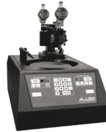
The **MultiPrep™ System** enables precise semiautomatic sample preparation of a wide range of materials for microscopic (optical, SEM, FIB, TEM, AFM, etc.) evaluation. Capabilities include parallel polishing, angle polishing, site-specific polishing or any combination thereof. It provides reproducible sample results by eliminating inconsistencies between users, regardless of their skill.
